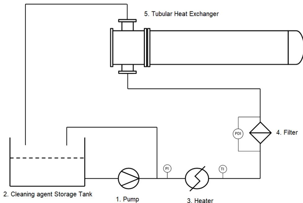
**Figure E-1—Example of tools and equipment for cleaning a tubular heat exchanger****E2 Cleaning agent selection**
